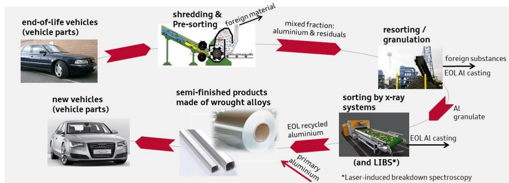
Figure 6. ALEOL project – development of a recycling process for recovering end-of-life aluminium wrought alloys from vehicle bodies.
